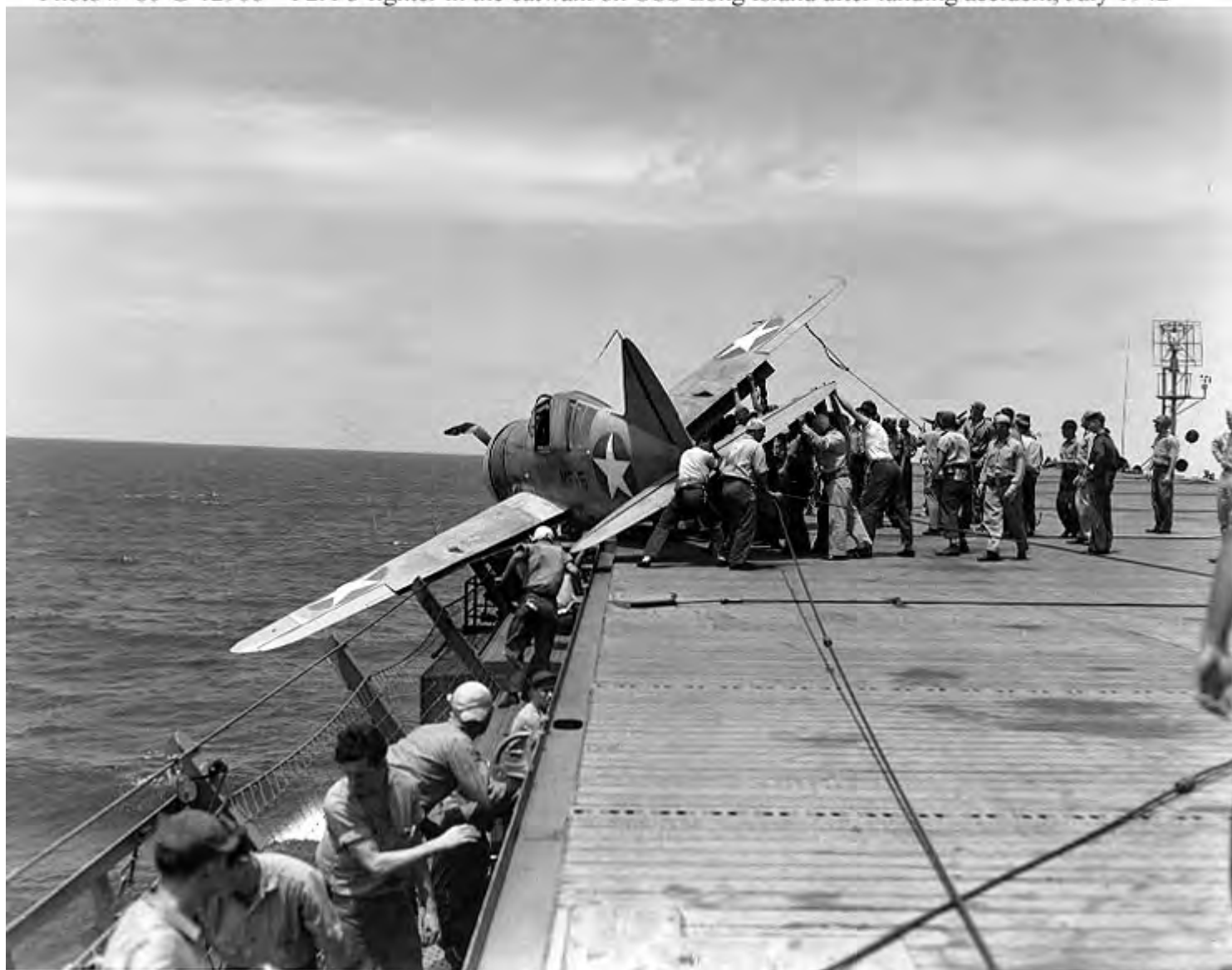
Photo # 80-G-12906 F2A-3 fighter in the catwalk on USS Long Island after landing accident, July 1942
